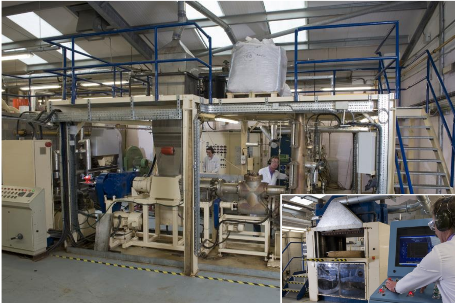
Pressurised refiner & hot press
