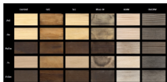
Figure 3: Colour change after exposure to different ageing procedures performed (OutDW-B is not included because the colour changes are similar to those of OutDW-A).
