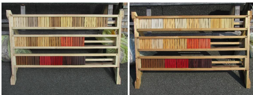
Figure 1: Weathering test of untreated and acetylated hornbeam coated with various oils and glazes, before (left) and after 31 days of exposure (right)
