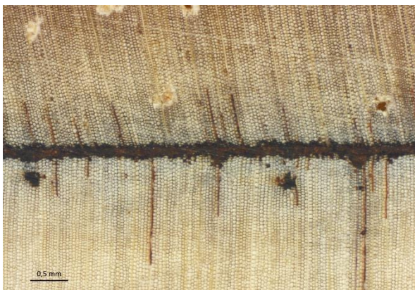
Figure 5: Glue line region of acetylated Radiata pine prepared by sanding; a PRF adhesive system was used in this samples
