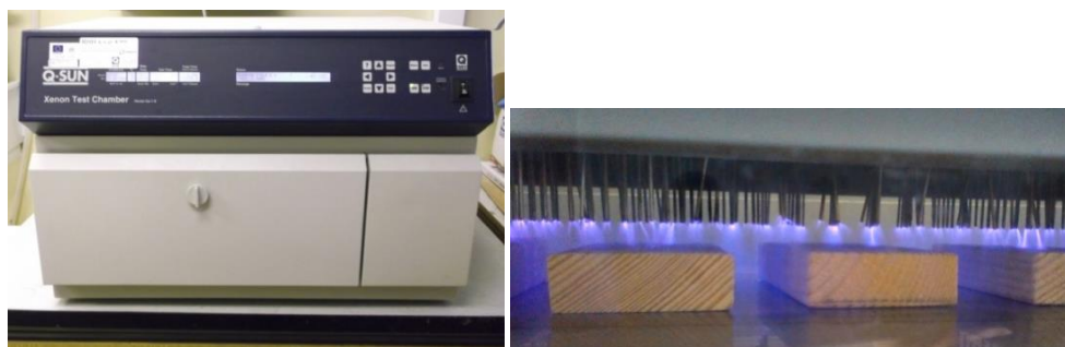
Figure 1: Plasma pre-treatment of the top surfaces of spruce samples in the ADRE device
