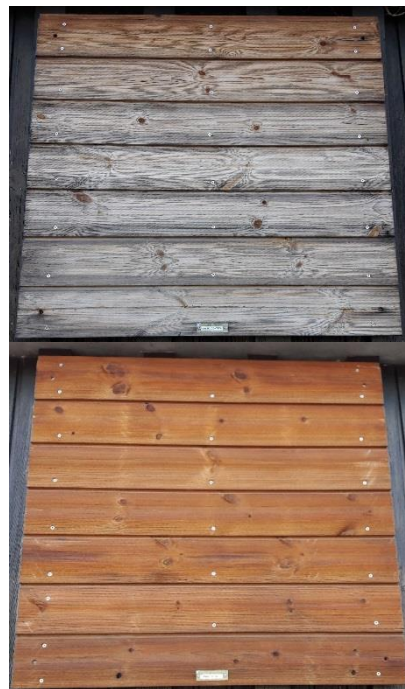
Figure 2: Non-treated ThermoWood reference (upper) and PF-treated ThermoWood (lower) outdoor weathering test elements after twenty months of outdoor exposure in Germany.
