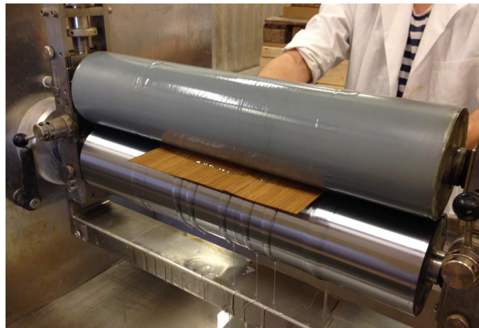
Figure 1: Roll pressing of an oak veneer sheet, coated with PEG 400. Excessive PEG (~ 50 %) dropping down.
