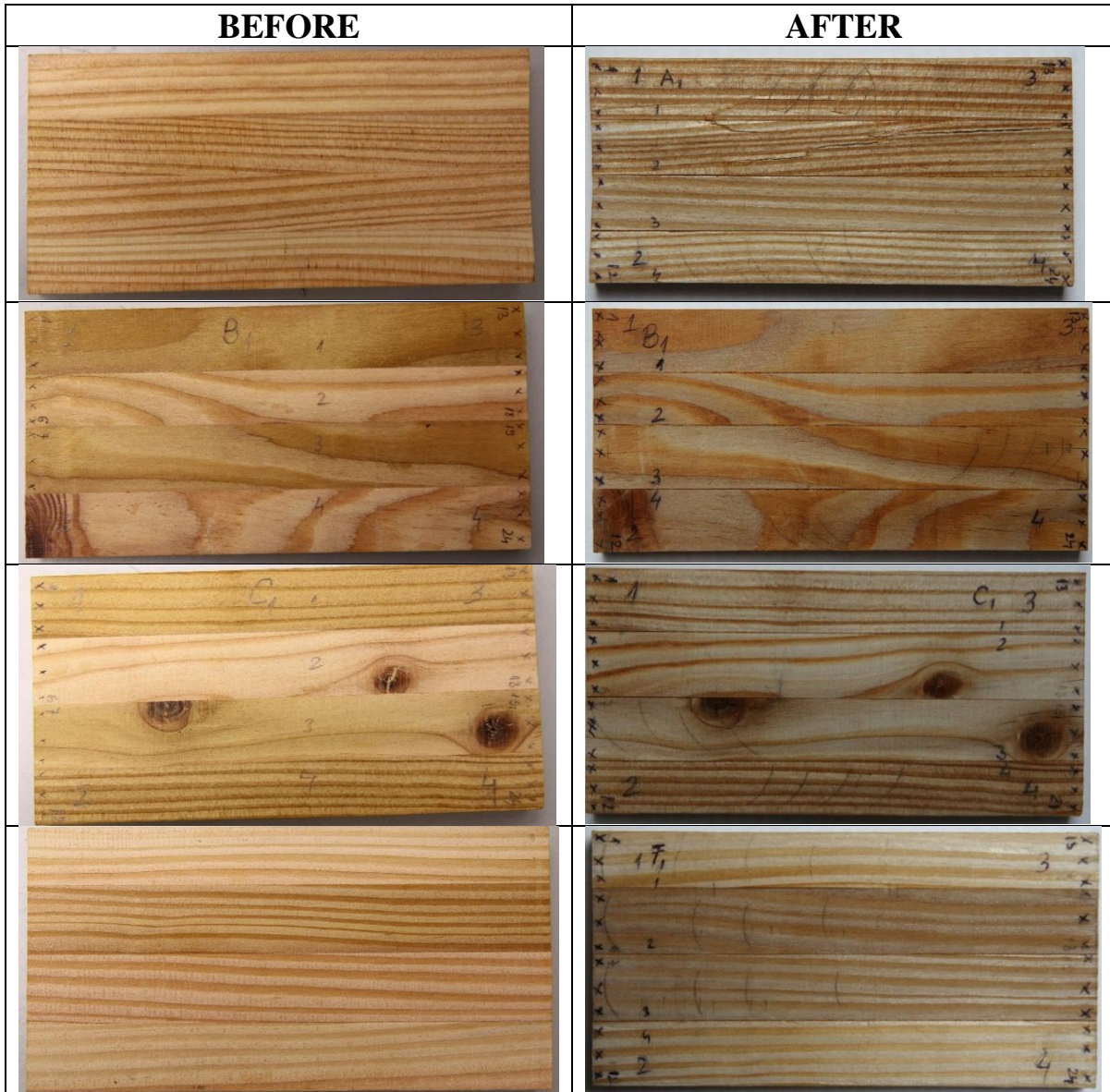
Figure 3: Photographs of samples A1b, B1b, C1b and F1b before and after QUV weathering exposure
