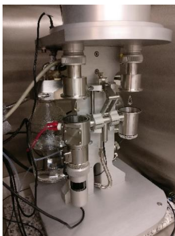
Figure 2: DVS apparatus opened for sample replacement
