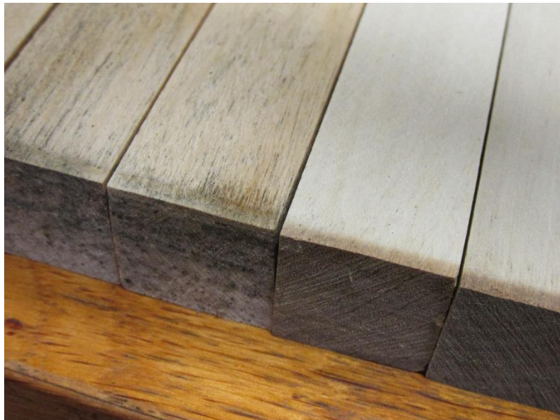
Figure 3: During the weathering test, untreated hornbeam was cracked and was attacked by mould (left) while acetylated hornbeam remained unharmed (right)
