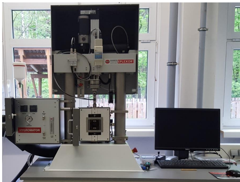
Figure 2: DMTA device “Eplexor 25” equipped with a humidity generator.
