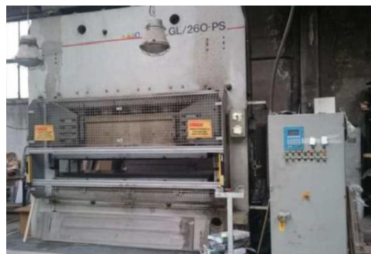
Figure 2: Press for wood densification, Italpress (model GL/260-PS)
