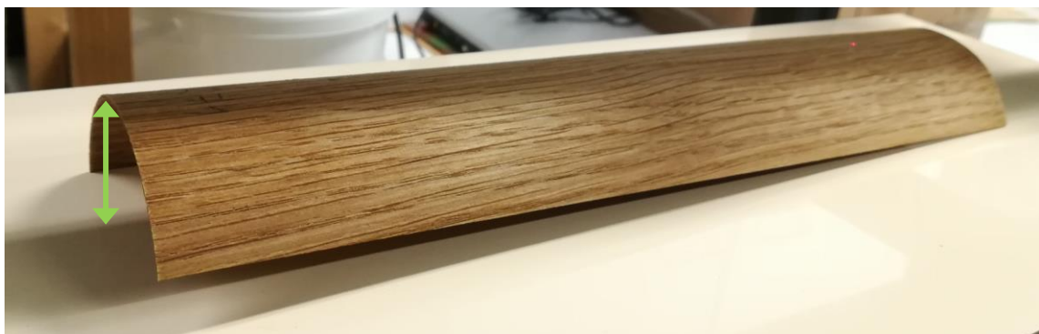
Figure 3: Deformation of oak veneer, 1 week after treatment. Upper side treated with PEG 400. Red dot indicates laser aided deformation measuring. Green arrow: lift distance as deformation indicator.
