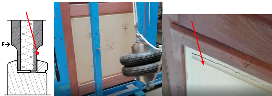
Figure 10: impression of a typical insulated, panel infill construction, with moulded edge profile. In a dynamic burglary resistance test (EN 1629)
