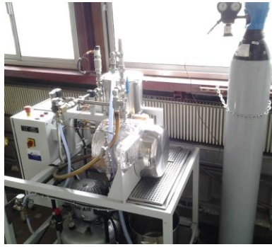
Figure 1: Autoclave for vacuum-pressure impregnation and thermal treatment
