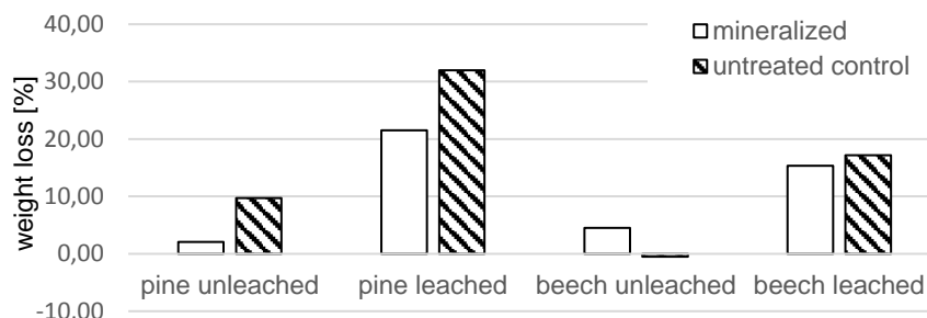
Figure 4 Weight loss of leached and unleached mineralized pine, and their untreated control caused by Coniophora puteana and weight loss of leached and unleached mineralized beech and their untreated control caused by Coriolus versicolor
