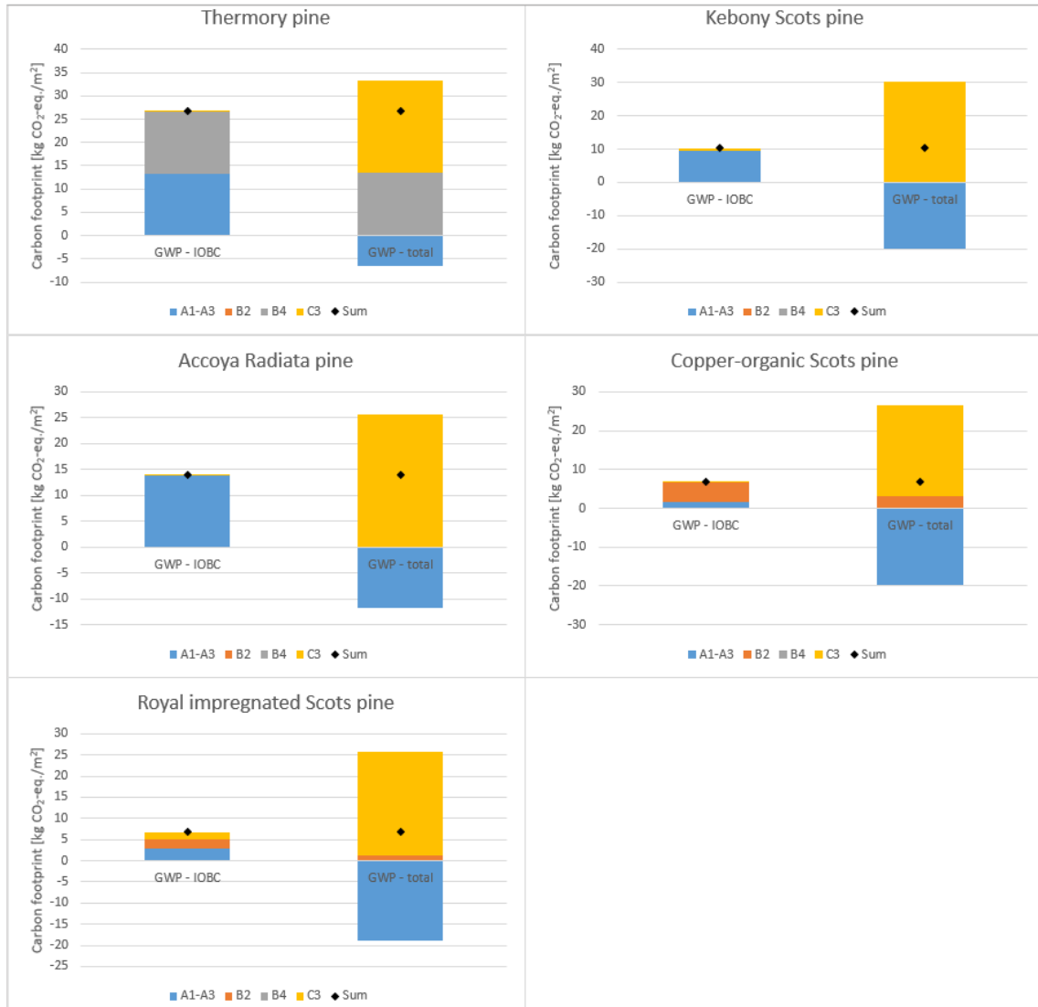
Figure 3: Results of the contribution analysis of each life cycle module A1-A3 = production of the materials, B2 = maintenance, B4 = replacement, C3 = waste treatment.
