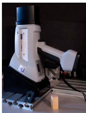
Figure 1: ED-XRF equipment used
