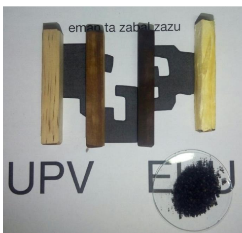
Figure 1: Visual aspect of the different woods, from left to right: untreated wood, heat-treated wood, weathered heat-treated wood, organosolv extracted wood and bleached wood.
